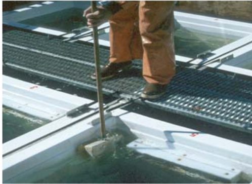
Picture 3a. The first step in cleaning the culture chamber is brushing the sides before the chamber is removed for cleaning.
