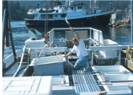
Picture 3b. Lifting the culture chamber from its housing. Notice that the elastic bungee chords must be removed before lifting.
