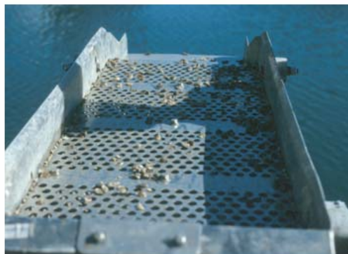
Picture 2e. Seed sorter with a 5/8" removable sorting plate. The plate vibrates with a reciprocating gear causing small seed to fall through the plate and larger seed move off the end at the top of the picture.
