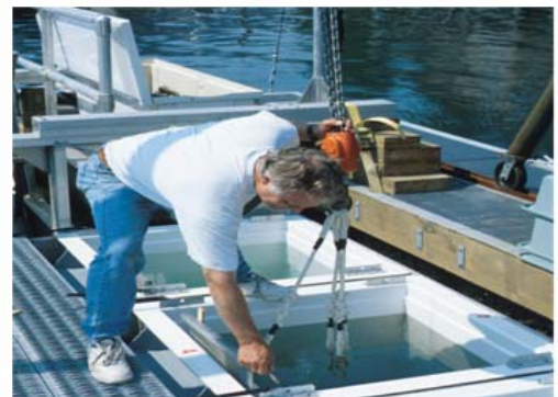
Picture 2f. Attaching bridle from the overhead hoist to the four corners of the culture chamber for lifting by the hoist.
